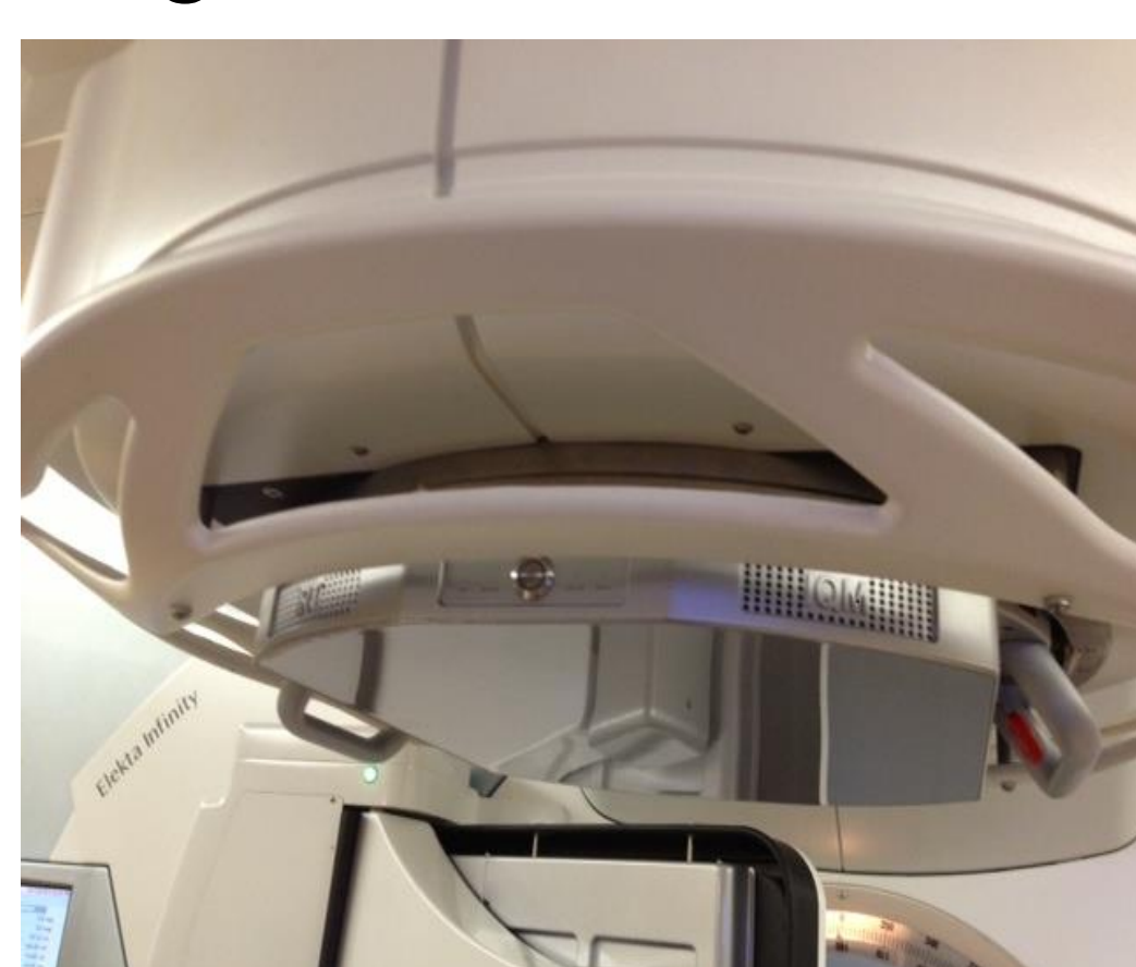
Figure 1. View of IQM mounting on the gantry
